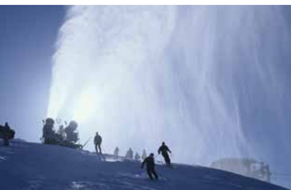
Snow-making machines spray water droplets into the air which freeze and become snow.
